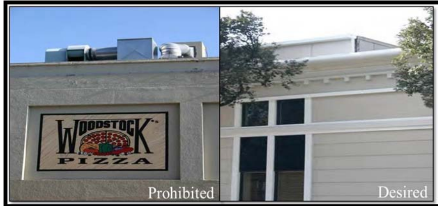
Figure 15.3-22. Rooftop Utilities Screening
